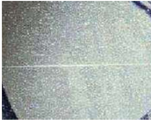
Fig. 1. Sliver defect on Al sheet after anodic oxidation (10 x)
