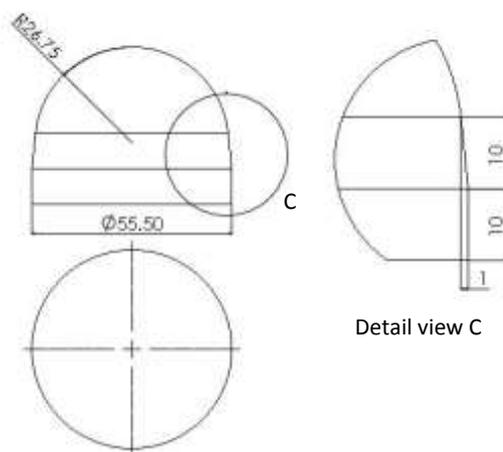
Fig. 7 Drawing of punch
