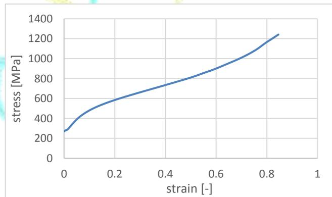
Fig. 3 Deformation resistance obtained from experiments
