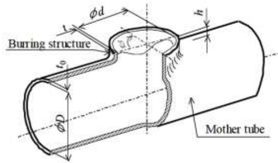
Fig. 1 Overview of branch pipe [2]
