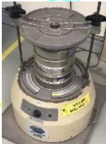
Figure 1: Dry sieve analysis equipment
