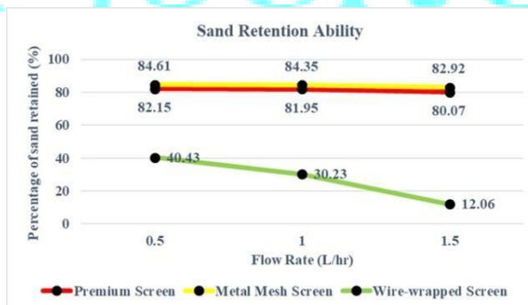
Figure 6: TC Sand Retentive Ability of Premium Screen, Metal Mesh Screen, and Wire-Wrapped Screen.
