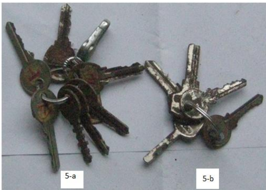
Figure 5. Rusty keys boiled with water; compare 5-a and 6-a; 5-b and 6b
