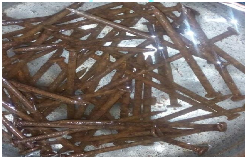
Figure 4. Rust nails boiled with water
